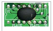
Chip on Board construction where the integrated circuit is created right on the circuit
